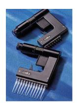
Corning offers 8- and 12channel adjustable 200µL micropipettors that are ideal for working in 96 well plates.
