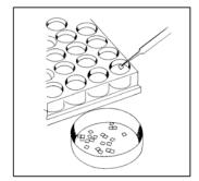
Figure 1. It takes a steady hand to pick up the glass chips and is initially quite challenging. But with practice it is possible to find and remove chips quickly and efficiently.
