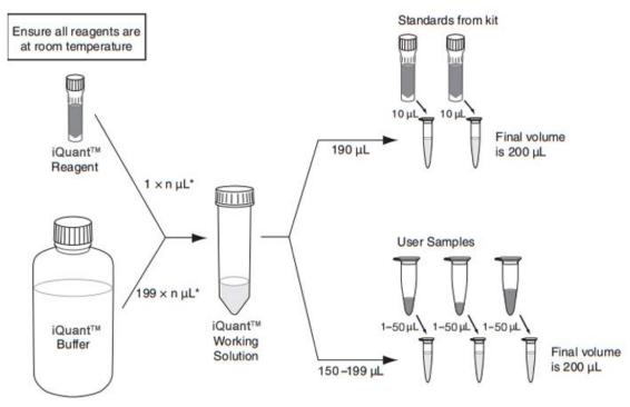
Figure 4. iQuant™ HS RNA quantitation assay workflow
